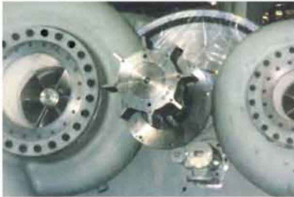
Compressor drives. Coupling mounted between electric motor and compressor input shaft.
